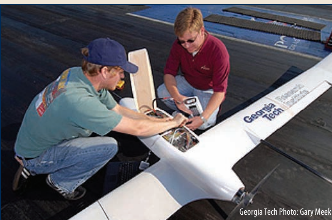
Thomas Bradley and Reid Thomas go through the procedure of starting up the fuel cell aircraft during a test flight at the Atlanta Dragway.
