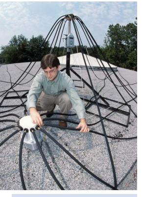
GTRI researchers are studying whether developing tornadoes emit very low-frequency sounds that could give forecasters an early detection method. Shown installing test equipment is Paul Hultz, a graduate student.
