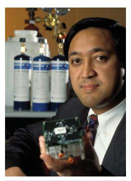
Hybrid electrical power sources composed of fuel cells, batteries, and capacitors could help meet unique military needs for sustained power, longterm power storage, and bursts of peak power. David Parekh, director of the Center for Innovative Fuel Cell and Battery Technologies, shows a GTRI-developed hybrid system.
